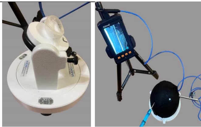
Figure 2: 3d printed labrum, glenoid base, and fully assembled L-CASTT
